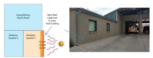
**Goal**: Apply ACS CIC 4.0 to exterior wall of sleeping quarter 1 to block solar heat loading to allow the thermostat to be set higher and make all 3 rooms more comfortable.
